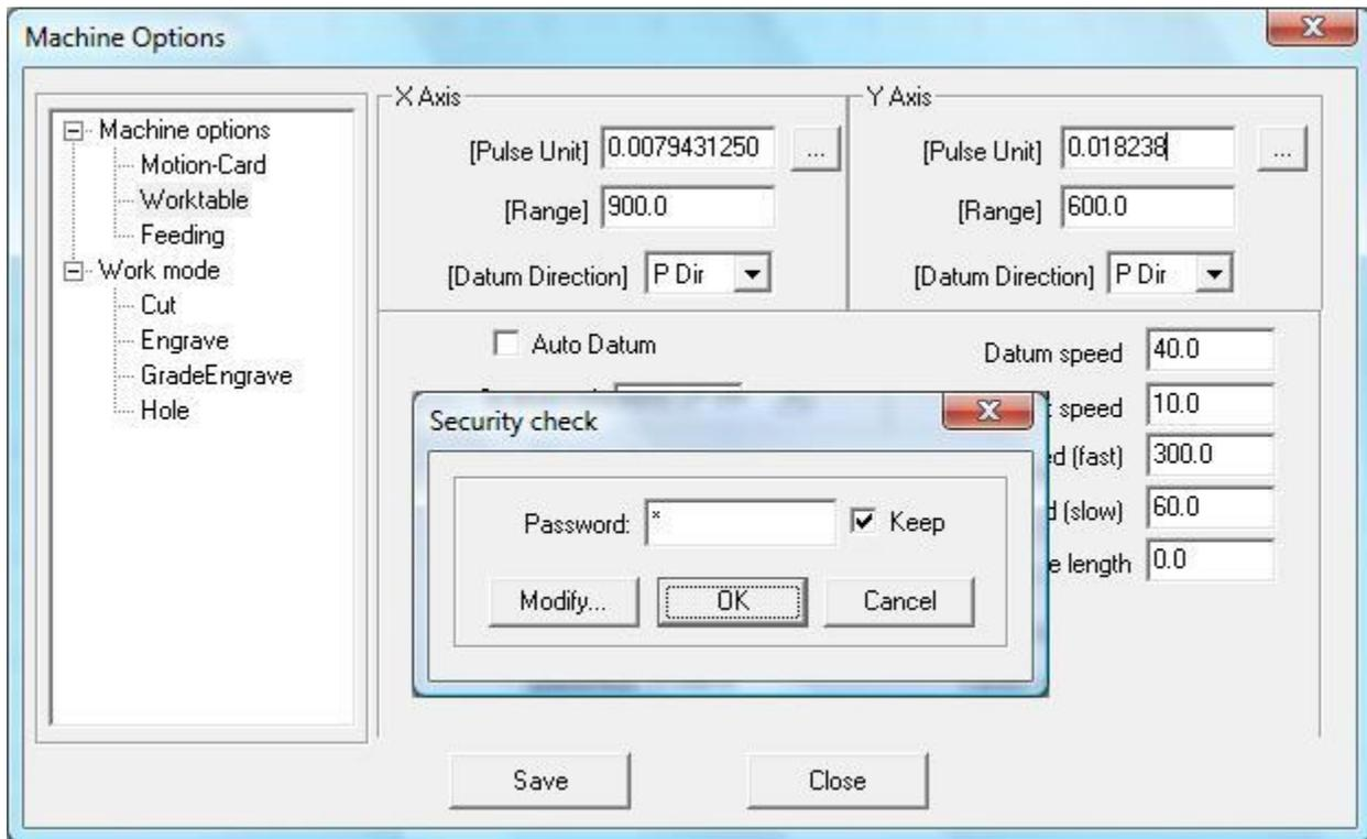
11) Save the changes to the "Machine Options" that we have just made. Simply press "OK" .. you should not need to insert a new password.
