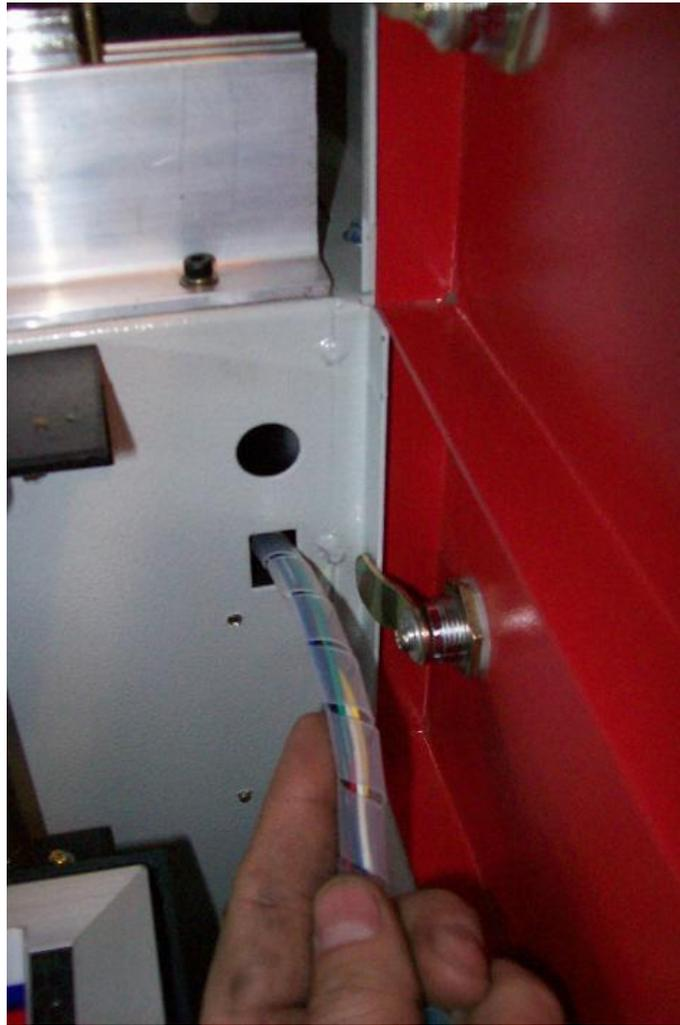
6) Now that the rotary attachment is sitting in place, it needs to be connected to the machine. The motor connector and wires need to be routed through the square hole and taken to the motor amplifier. This picture shows the square hole from inside the laser work area.
