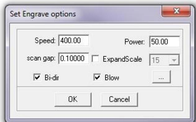
The final step in using the modified air assist system is to enable the software. The software features settings for enabling the “Blow Signal” during the lasering process. These selectable checkboxes can be found in the dialog boxes when setting the options of the Cut, Engrave, Grade Engrave, or Holes feature of each color layer.
